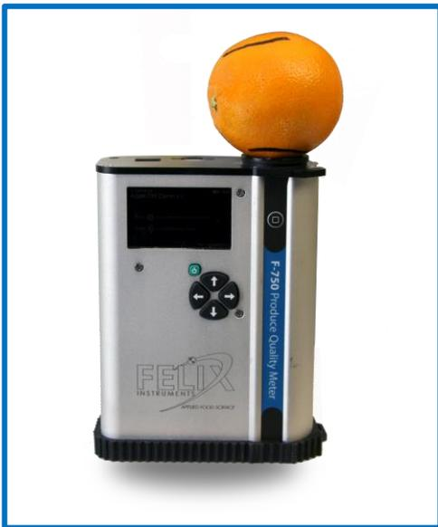
Figure 1. F-750 in the process of measuring oranges.
