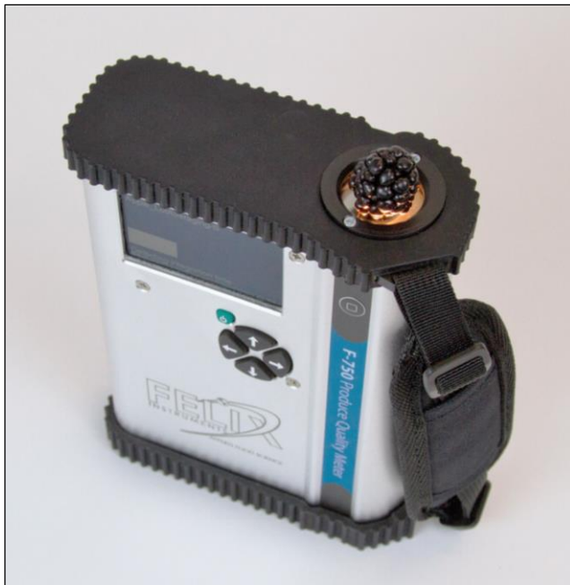
Figure 1. Fruit presentation for measuring blackberries with the F-750.
